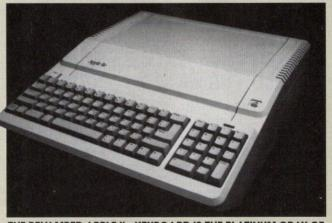
THE REVAMPED APPLE IIE KEYBOARD IS THE PLATINUM GRAY OF THE IIGS AND HAS A NUMERIC KEYPAD.
